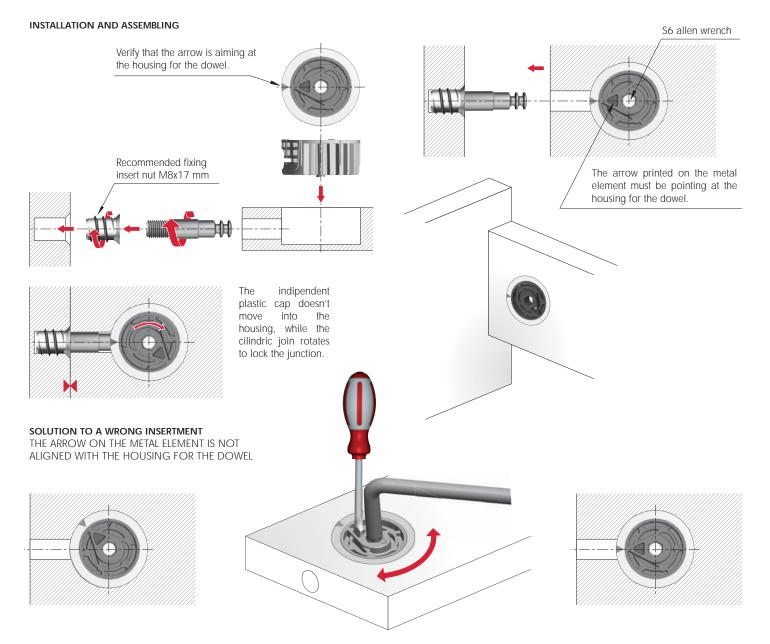
Rotate the connecting fitting with a S6 hexagonal key until the metal arrow and its matching point on the plastic cap are aligned.
